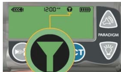
Sensor is “ON’ but not communicating with pump.
